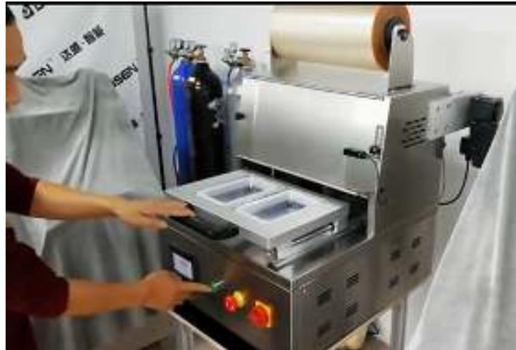
**Figure 2.1 Modified Atmosphere Sealer Packaging Machine**
