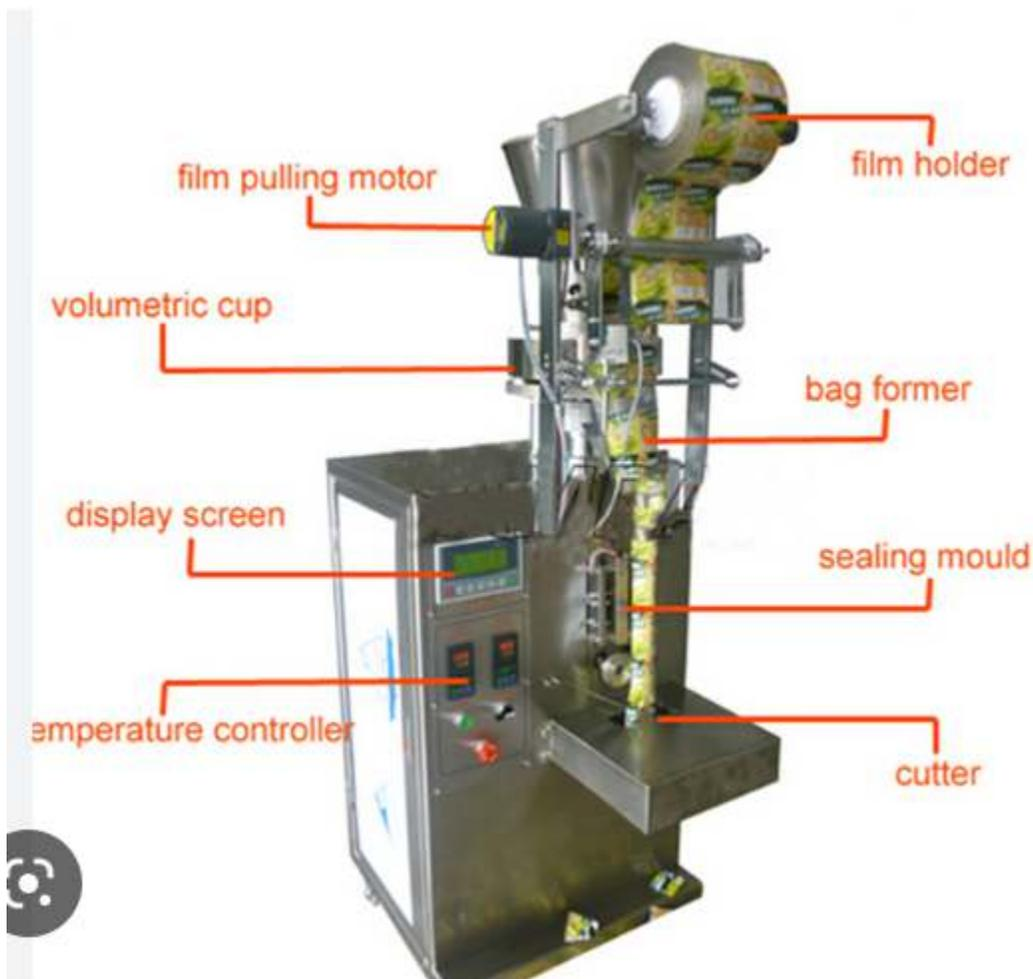
Figure 1.12: Vertical filling machine
