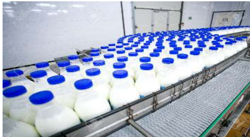
Figure 2.14 Food conveying systems in the plant
