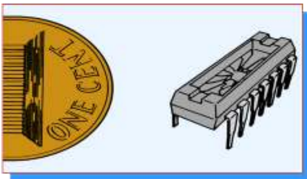
Figure: 3.1 Contains microscopic diodes, transistors, resistors, and capacitors in a wafer-like chip
