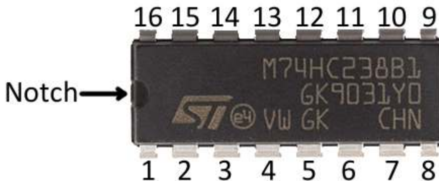
Figure 2.9: Polarity and pin numbering of ICs
