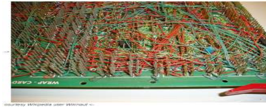
Figure 1.7: Printed circuit board wire wrapping
