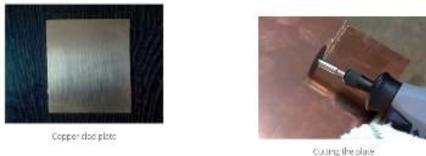
Figure 2.32 cut the copper board
