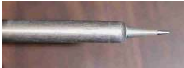
Figure 2.53.A properly cleaned and “wetted” soldering iron tip.
