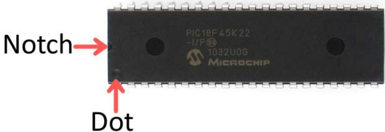
Figure 2.8: Polarity and pin numbering of ICs
