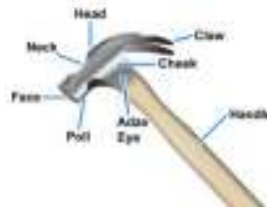
Fig.2.2. Parts of a claw hammer
