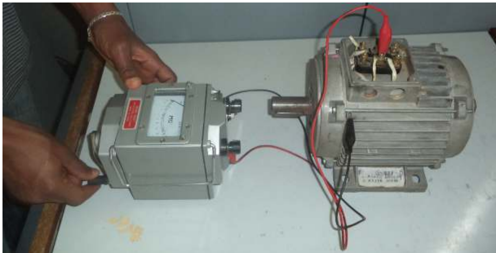
Figure 3.12 insulation resistance testing
