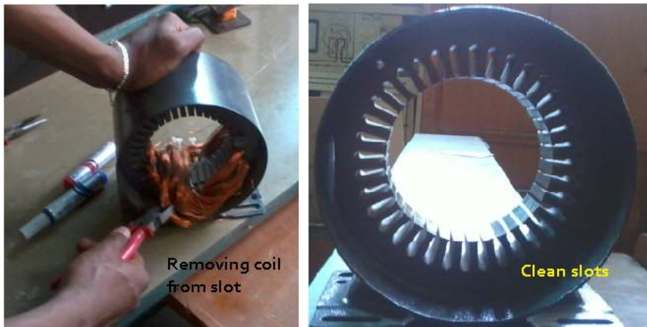
Figure 3.2 removing burn out coil
