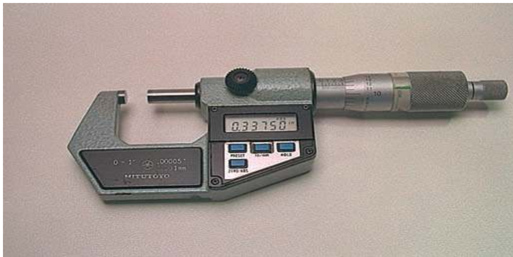
Figure2. 7 A digital micrometers eliminates the need to do math.
