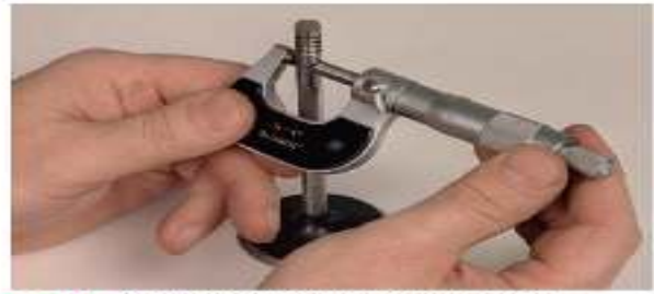
P2-8 To get an accurate reading, slowly close the micrometer until a slight drag is felt while passing the valve in and out of the micrometer.
