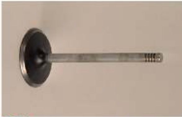
P2-1 Micrometers can be used to measure the diameter of many different objects. By measuring the diameter of a valve stem in two places, the wear of the stem can be determined.
