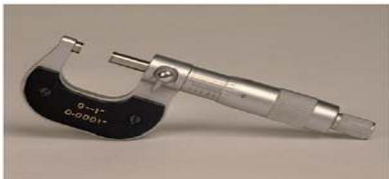
P2-5 A micrometer reading of 0.500 inch.
