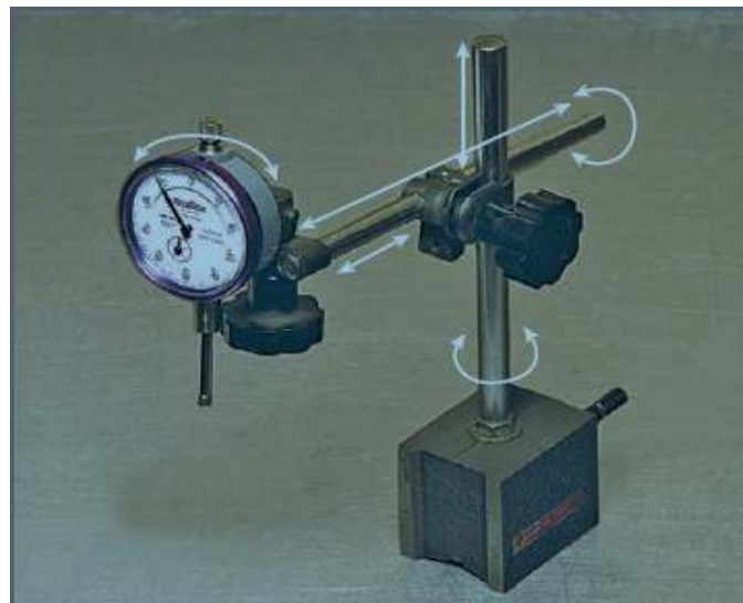
Figure2. 18 A dial indicators with a highly adaptive holding fixture.
