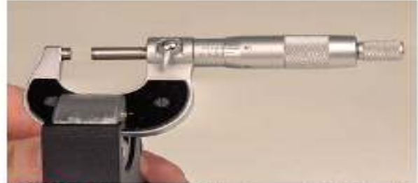
P2-10 This reading (0.311 inch) represents the diameter of the valve stem at the top of the wear area.
