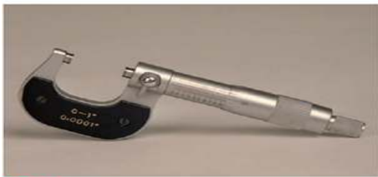
P2-3 The graduations on the sleeve each represent 0.025 inch. To read a measurement on a micrometer, begin by counting the visible lines on the sleeve and multiplying them by 0.025.
