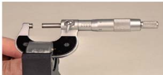
P2-6 A micrometer reading of 0.375 inch.
