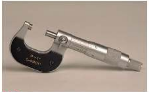
P2-2 Because the diameter of a valve stem is less than 1 inch, a 0-to-1-inch outside micrometer is used.
