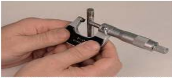
P2-7 Normally, little stem wear is evident directly below the keeper grooves. To measure the diameter of the stem at that point, close the micrometer around the stem.
