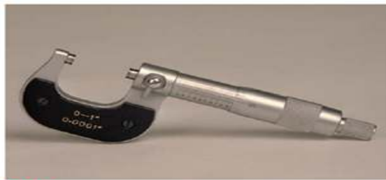
P2-4 The graduations on the thimble assembly define the area between the lines on the sleeve. The number indicated on the thimble is added to the measurement shown on the sleeve.
