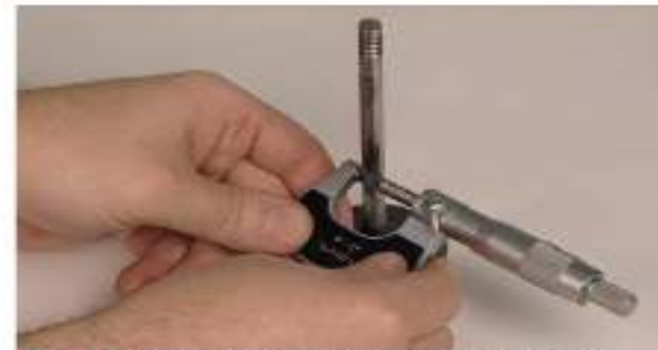
P2-12 Most valve stem wear occurs above the valve head. The diameter here should also be measured. The difference between the diameter of the valve stem just below the keepers and just above the valve head represents the amount of valve stem wear.
