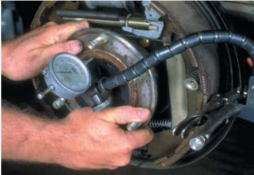
Figure2. 19 This dial indicator setup will measure the amount this axle can move in and out.
