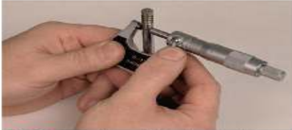
P2-9 To prevent the reading from changing while you move the micrometer away from the stem, use your thumb to activate the lock lever.
