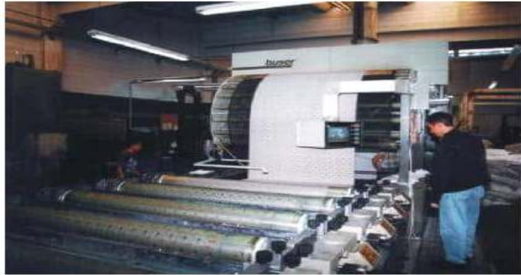
Fig 2.5. Cylinder or roller printing
