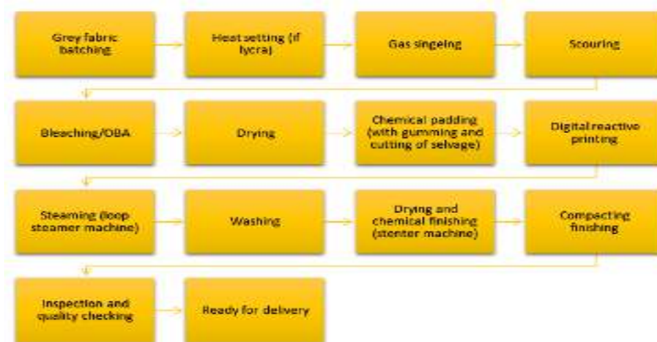
Fig 2.2. Process Flowchart for Digital Textile Printing
