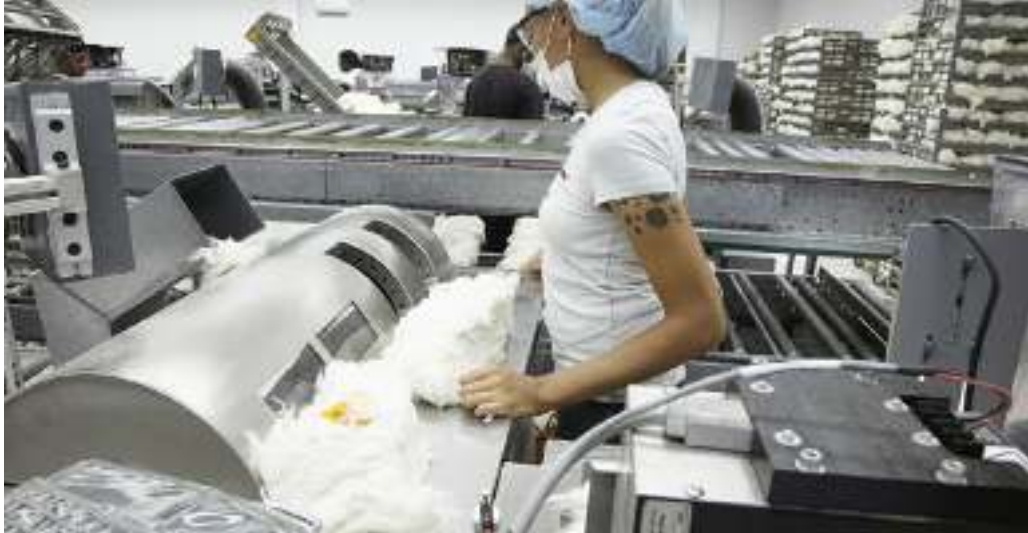
Fig3.3 Fiber length and strength measurements are made on the same “beard” of cotton.
