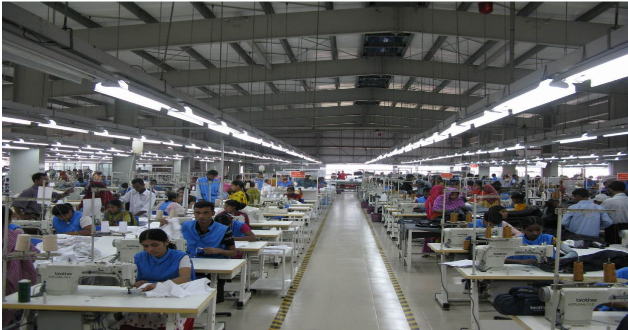
Fig: Progressive Bundle System
