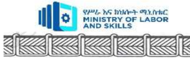
Fig :-3.1.4. Seam when the upper tension is too tight
