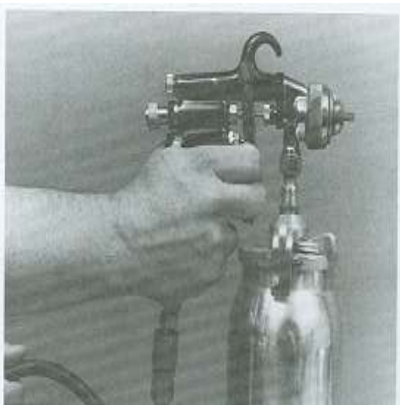
Suction feed type spray gun
