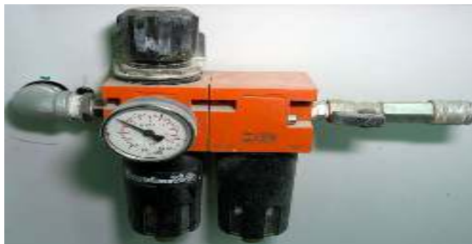
Fig.1.6 Devil Bliss DVFR-2 Filter Regulator, Coalescer
