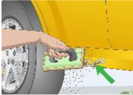
Fig: 2. Check for rust and remove any you find
