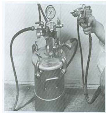
Pressure feed type spray gun
