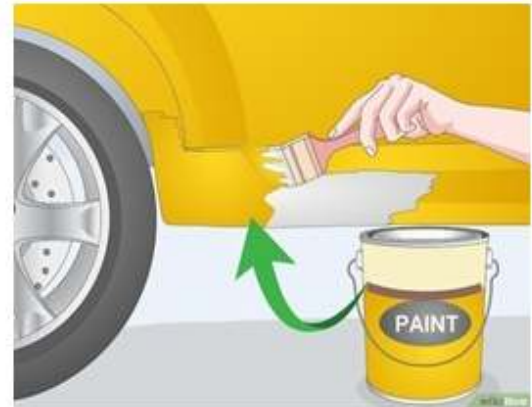
Fig: 6. Apply the touch-up paint to the primed area
