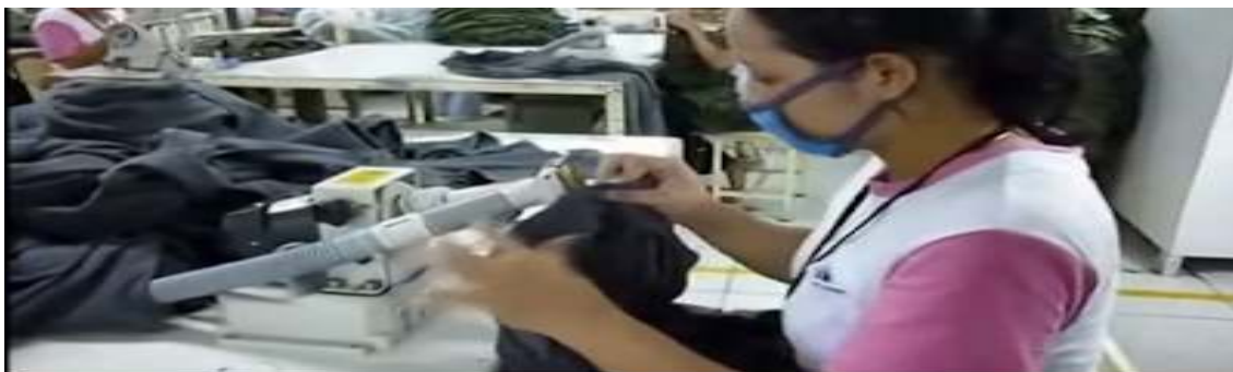
Fig2.2: Thread trimming machine (Unisun)
