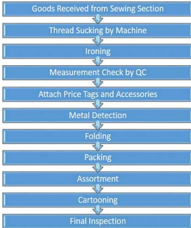
1.9 Flow chart of garments finishing
