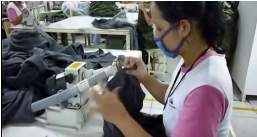
Fig1.3: Thread trimming machine
