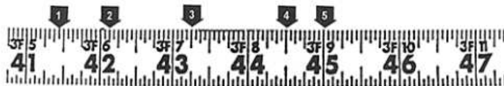
Figure 2.4 Consideration while measuring with tape
