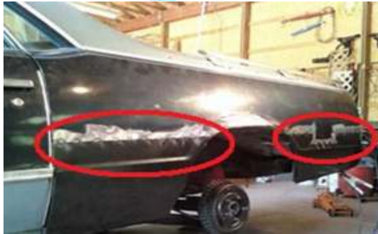
Figure1. 2: Welding prepared panel with vehicle body
