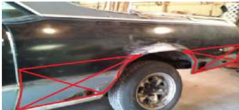
Figure1. 1: Selecting the Vehicle damaged part need to be repair
