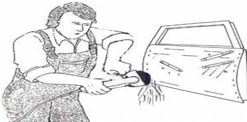
Figure 2.3.5 Grinding/Filing a Door Panel
