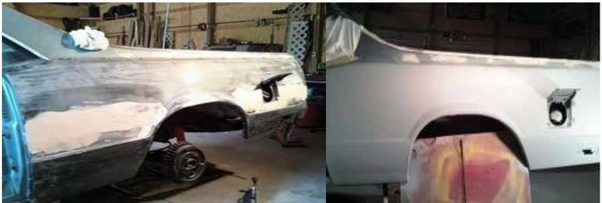
Figure1. 5: Sanding the Panel after applying putty
