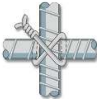
Fig.2.12. Crown tie, cross tie or figure-eight tie
