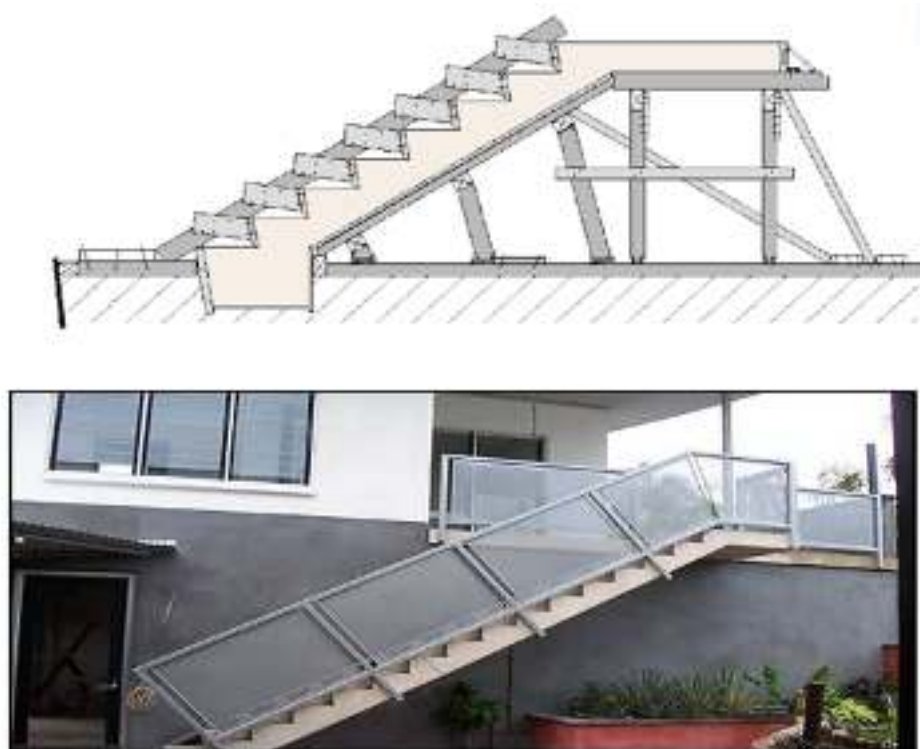
Fig.1.24. Steel stair formwork
