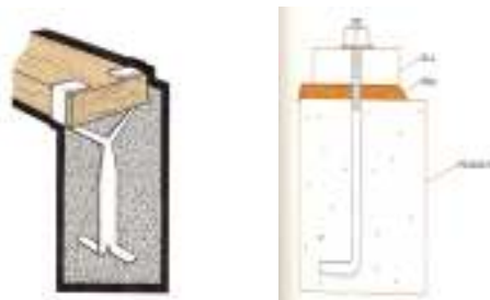
Figure 3.7 Anchor strap used to anchor the sill and Anchor bolt in foundation
