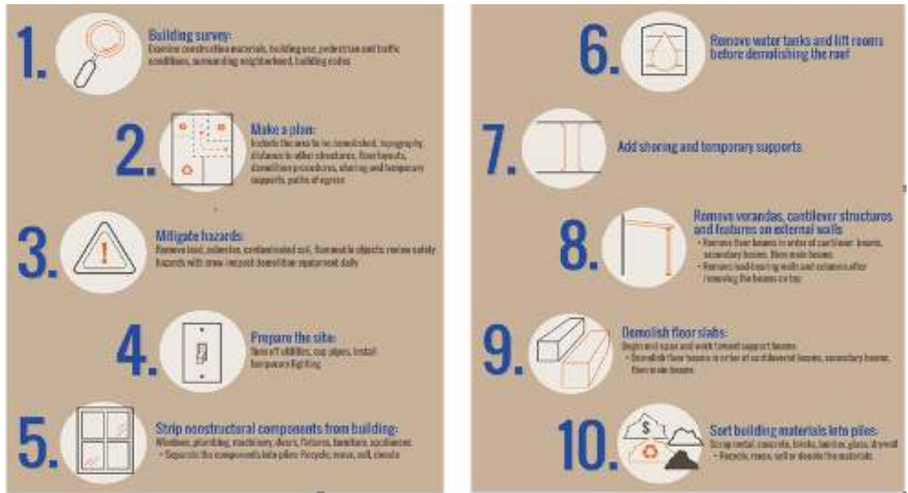
Figure 2.16 Procedures of demolition work
