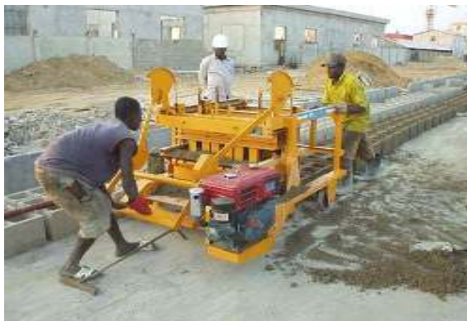
Fig.3.1 Block producing machine used to produce HCB
