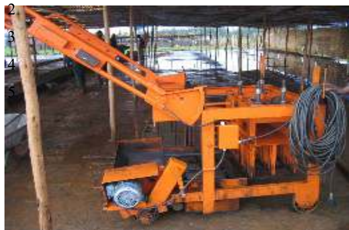
Fig.3.1 Block producing machine used to produce HCB
