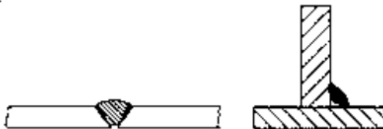
Figure: 4.5: Lack of Penetration
