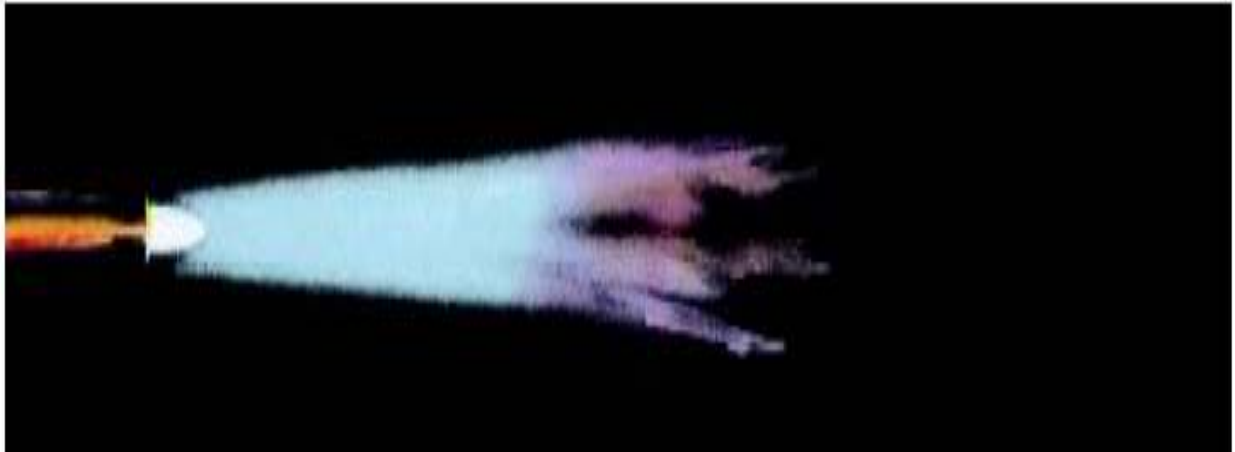
Figure.3.10. Oxidizing Flame (Acetylene and excess oxygen, 6300°F)
