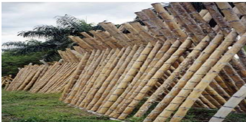
Figure 3: Oblique (Leaning piling) bamboo culms for open air drying
