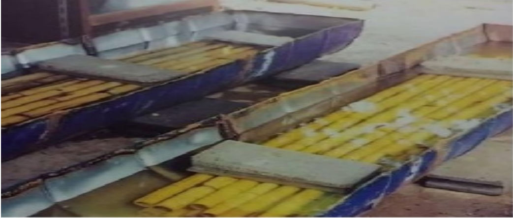
Figure1: Dipping water or chemicals for treatment
