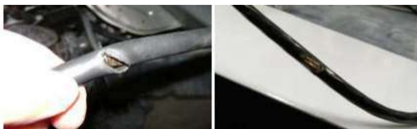
Figure 2.9 Look for tear/cut insulator
