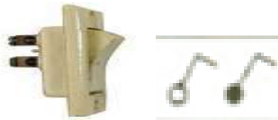
Figure 1.24 one way switch pictorial diagram and symbol
