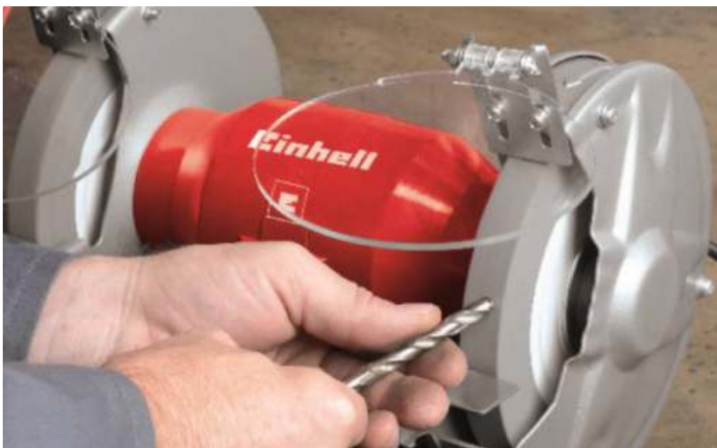
Figure 3.6 Drill bits sharpening.
