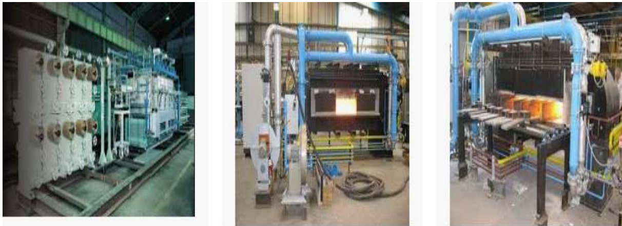
Figure 3.4 Slot type furnace
