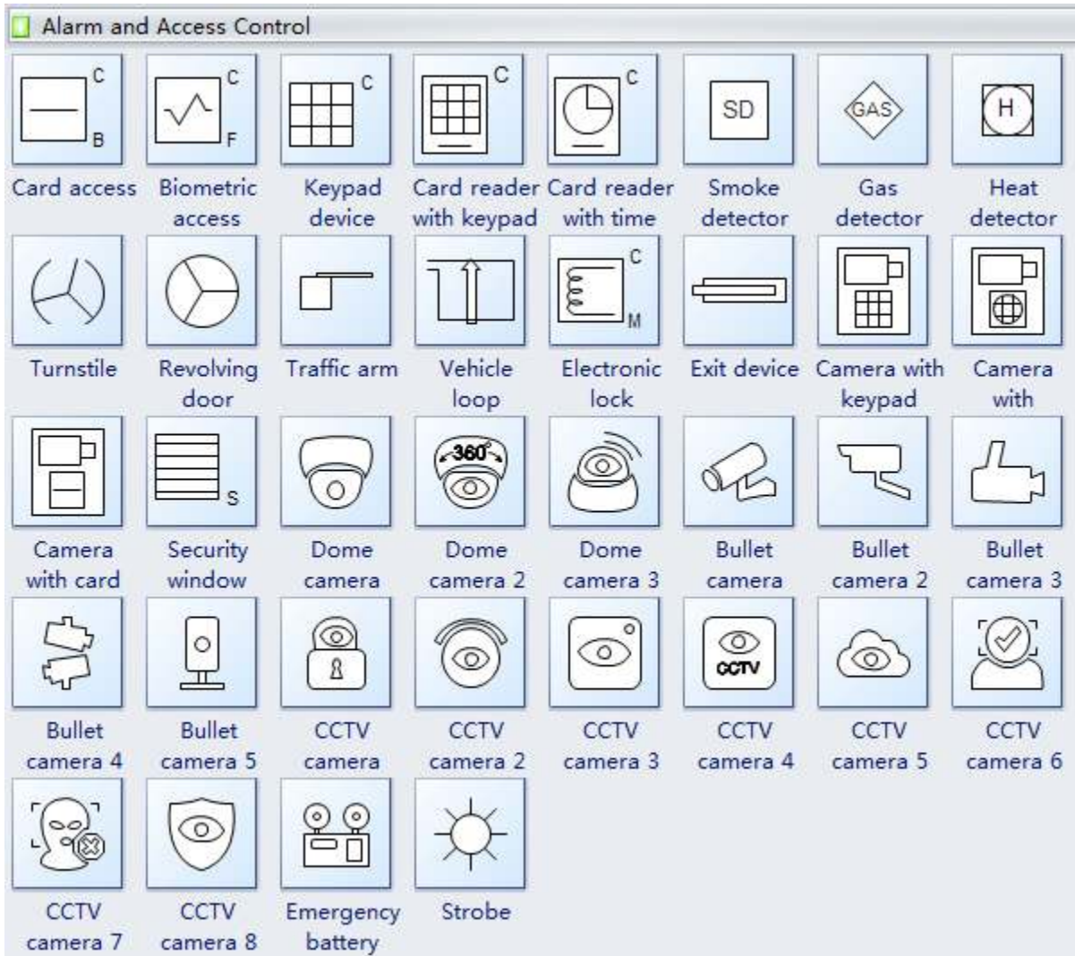
Fig 1.5.1 Comen symbol for alarm and access controle
