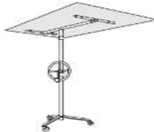
FIG:1.26. Panel Lift
