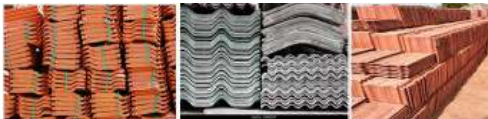
Fig 4.7 Storing of roof tiles
