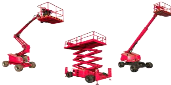
Figure 0-4 Elevating Work Platforms
