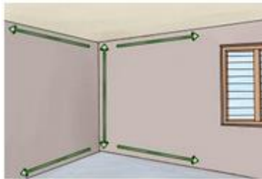
Figure4.9 cutting block plaster
