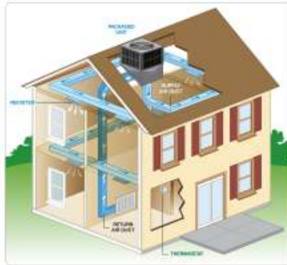
Fig 1.11: Packaged heating and cooling systems
