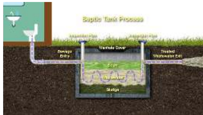
Figure 1-1 Septic tank systems
