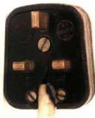
fig 6. Cracked casing and damaged cable sheath
