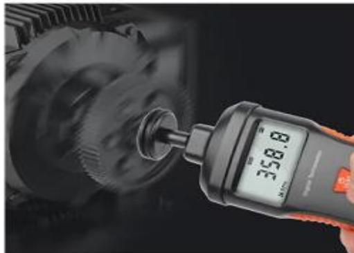
Fig19. Measure motor speed use Tachometer
