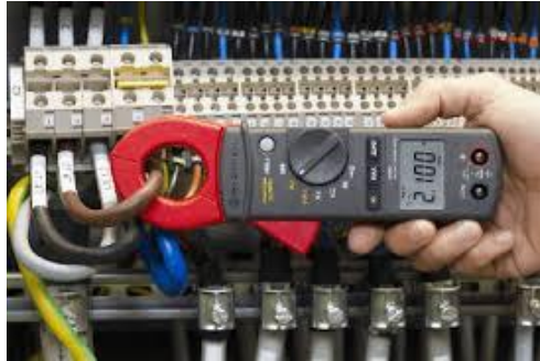
Fig16. Measure current use clamp meter
