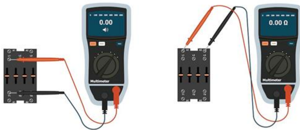
Fig. 2.12: Contactor terminal testing
