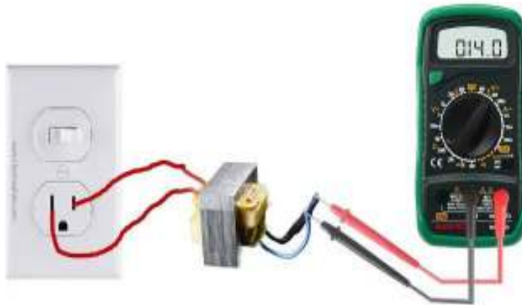
Fig 12. Test secundar voltage transformer
