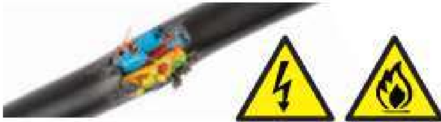
Figure4. 6 Risk occurs if 'live' conductor or broken conductor strands.
